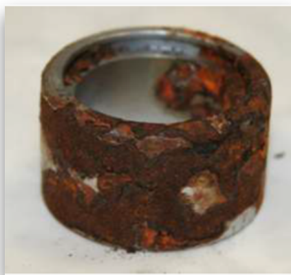
Figure 1 Competitor's Chrome Plated Bearing Steel Pre and Post Test
