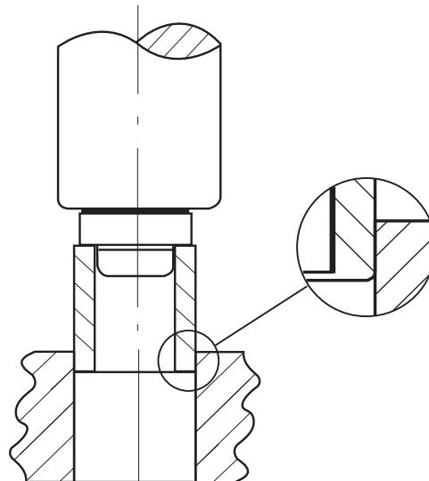
**FIGURE 12:** Journal bearing assembly tool
