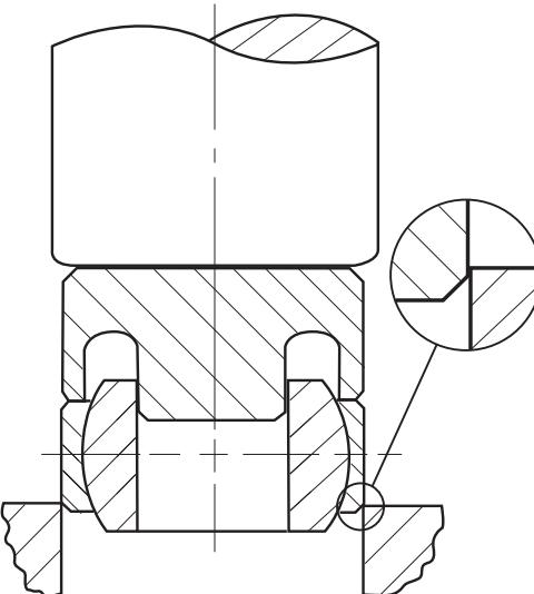
**FIGURE 11:** Spherical bearing assembly tool
