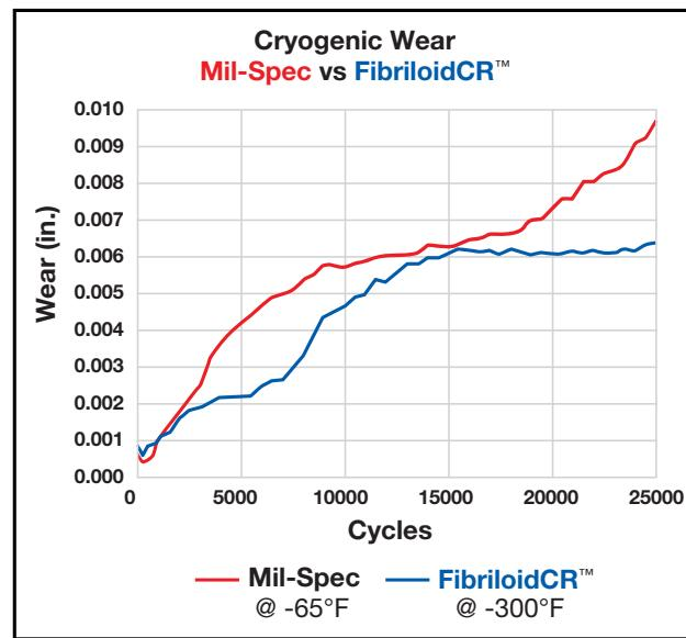
**Figure 1.** Test data from cryogenic oscillation under radial load, 40 ksi bearing stress, 20 cycles per minute,  $\pm 25^\circ$  angle of oscillation (Top) Coefficient of friction data; (Bottom) Wear data
