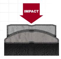
RBC ImpactTuff® Spherical Plain Bearings have a shock absorbing ductile core. This core absorbs impacts and impedes crack propagation through the ring.
