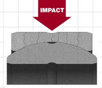
Excessive impact loads applied to "Thru-Hardened" Spherical Plain Bearings can lead to brittle fracturing of the rings.
