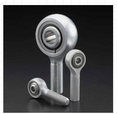
Heim® AeroCres® Ball Bearing Rod Ends are precision ground to tight tolerances for applications requiring self alignment, low torque and reduced radial clearance. They are greased and equipped with PTFE seals bonded to corrosion resistant caps.
