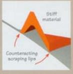
wanted to minimize lube loss with constant pressure on the inner sphere while maximizing lube replacement efficiency.
