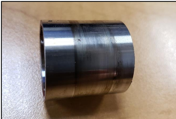
Figure 6. PTFE transfer film burnished onto a counterface bushing
